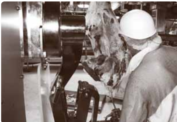
The HookAssist technology enables easier handling of the beef carcase
